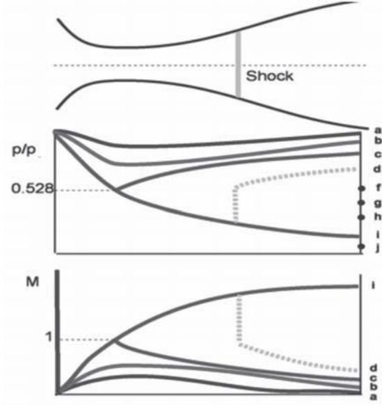
Fig. 1 Flow through Convergent Divergent Nozzle
