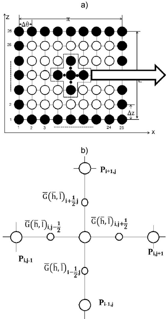
Fig. 2: Separation of the set of nodal points for the finite difference method from the surface of the bearing a) Schematic drawing showing the grid points used b) view of a single set of five adjacent points
