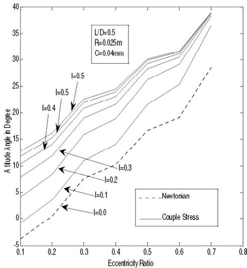
Fig.3 Attitude angle vs. eccentricity at different couple stresses parameter
