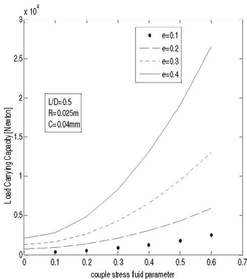
Fig.4 Load carrying capacity vs. non-dimensional couple stresses parameter
