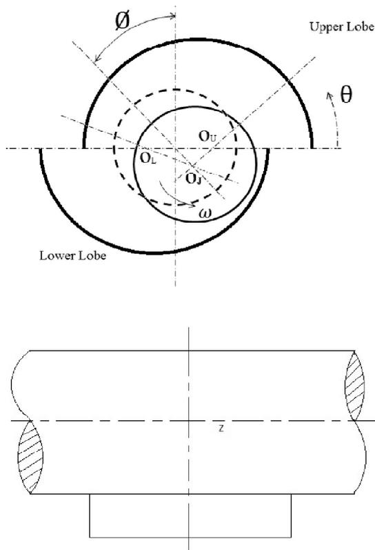
Fig.1 Physical configuration of an offset journal bearing
