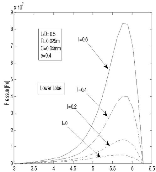
Fig.5 Effect of couple stress fluid parameter on pressure profile of the lower lobe of offset journal bearing
