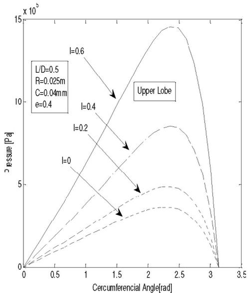
Fig. 6 Effect of couple stress fluid parameter on pressure profile of the upper lobe of offset journal bearing. Fig.4 shows the dimensionless load capacity as a function of couple stress parameter for different values of eccentricity ratio for aspect ratio=0.5. It can be seen from this figure that load carrying capacity is enhanced with increase in couple stress parameter and eccentricity ratio. Hence, journal can sustain more loads for couple stress fluid than Newtonian fluid.
